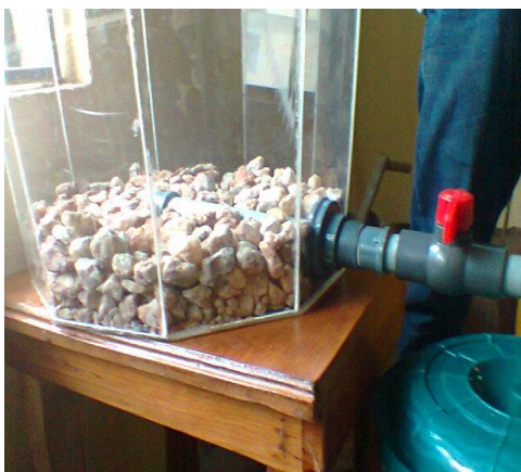
Fig.1: Slow sand water filter
