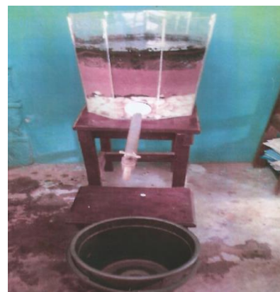
Fig. 2: Slow sand filter with activated carbon
